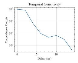
Unlike the first experiment, we have a strong peak at no delay, suggesting that the two photons are correlated which makes sense since they originate from just 1 photon.
