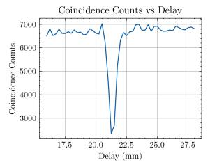
window. This point corresponds to the point where the two photons are indistinguishable. When this occurs, the photons have correlated behavior. In this case, the bunch together and leave out the same port as shown situations (c) and (d). However, when one photon is delayed, it is possible to distinguish them based on their respective paths by inferring from the arrival times.
